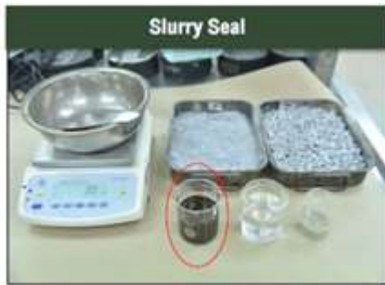
Exhibit 19: Mixing test for asphalt slurry seal
