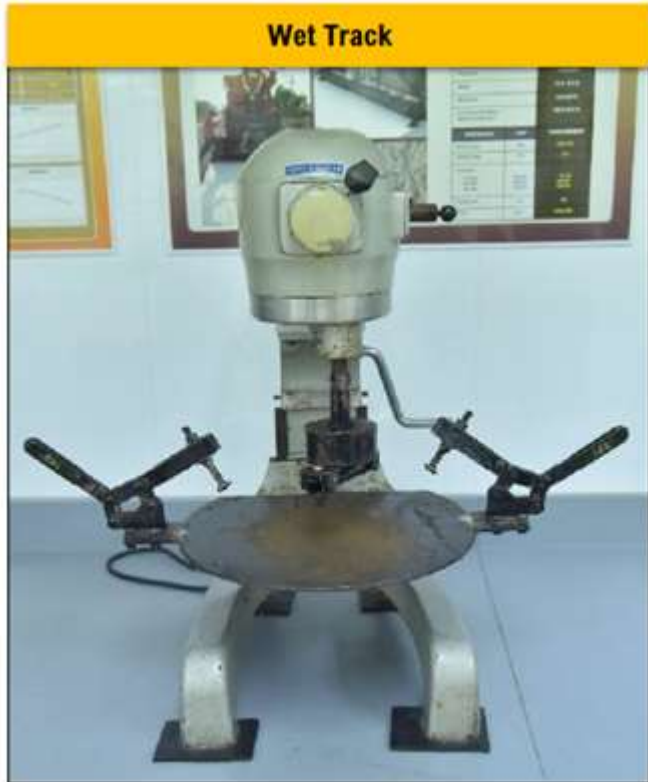
Exhibit 23: Wet track abrasion test (slurry seals vs para slurry seal)
