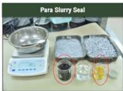
Exhibit 21: Mixing test for premium asphalt para slurry seal
