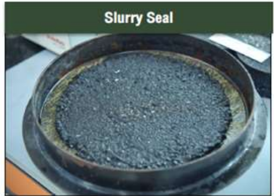
Exhibit 24: Premium para slurry seal asphalt has a higher water resistance than slurry seal
